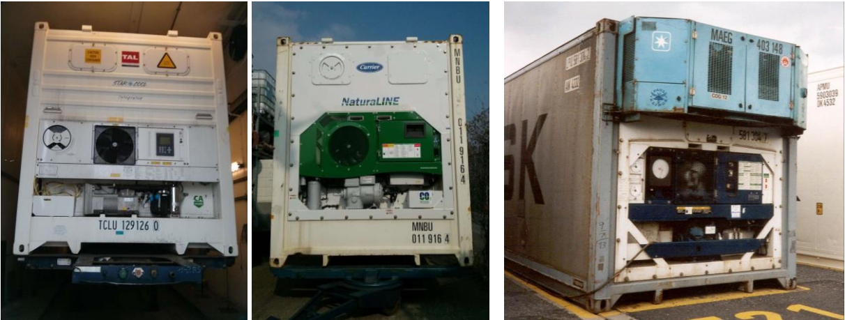
Temperature-controlled integral containers 14
