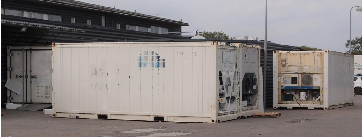
Figure 11. 20 feet reefers used permanently as extended refrigerated storage room at food wholesaler
