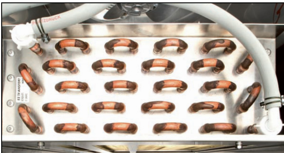
Figure 9 Heat exchanger of a flight-type dishwasher
