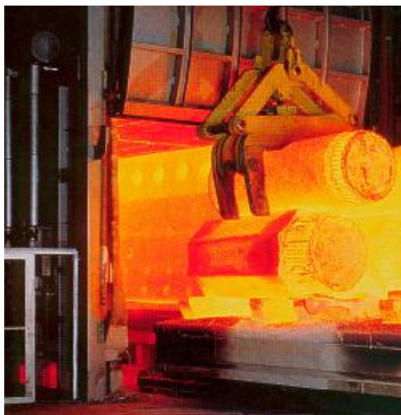
Figure 11. Batch foundry furnace for heating large steel parts
