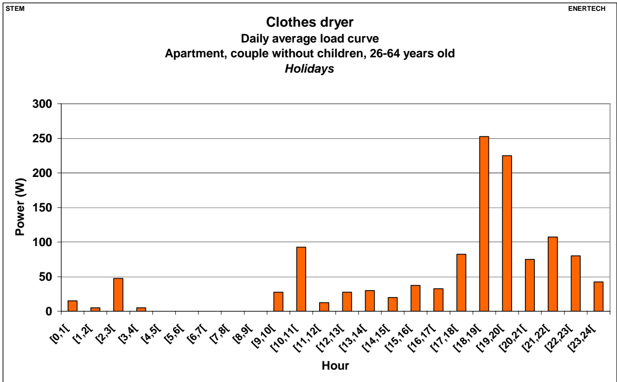
Figure 2.238: Clothes dryer – Daily average load curve – Apartment, couples without children, 26-64 years old – Holidays
